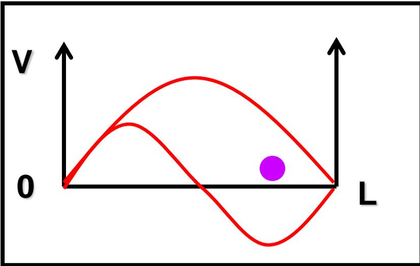
$$V(x) = \begin{cases} 0, & \text{for } 0 < x < L \\ \infty, & \text{for } x < 0 \text{ and } x > L \end{cases}$$
